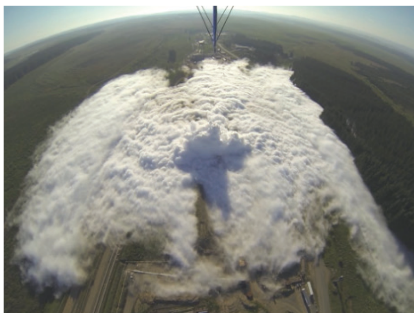
CO 2 cloud from a rupture test performed at DNV GL Spadeadam, Photo: DNV GL
